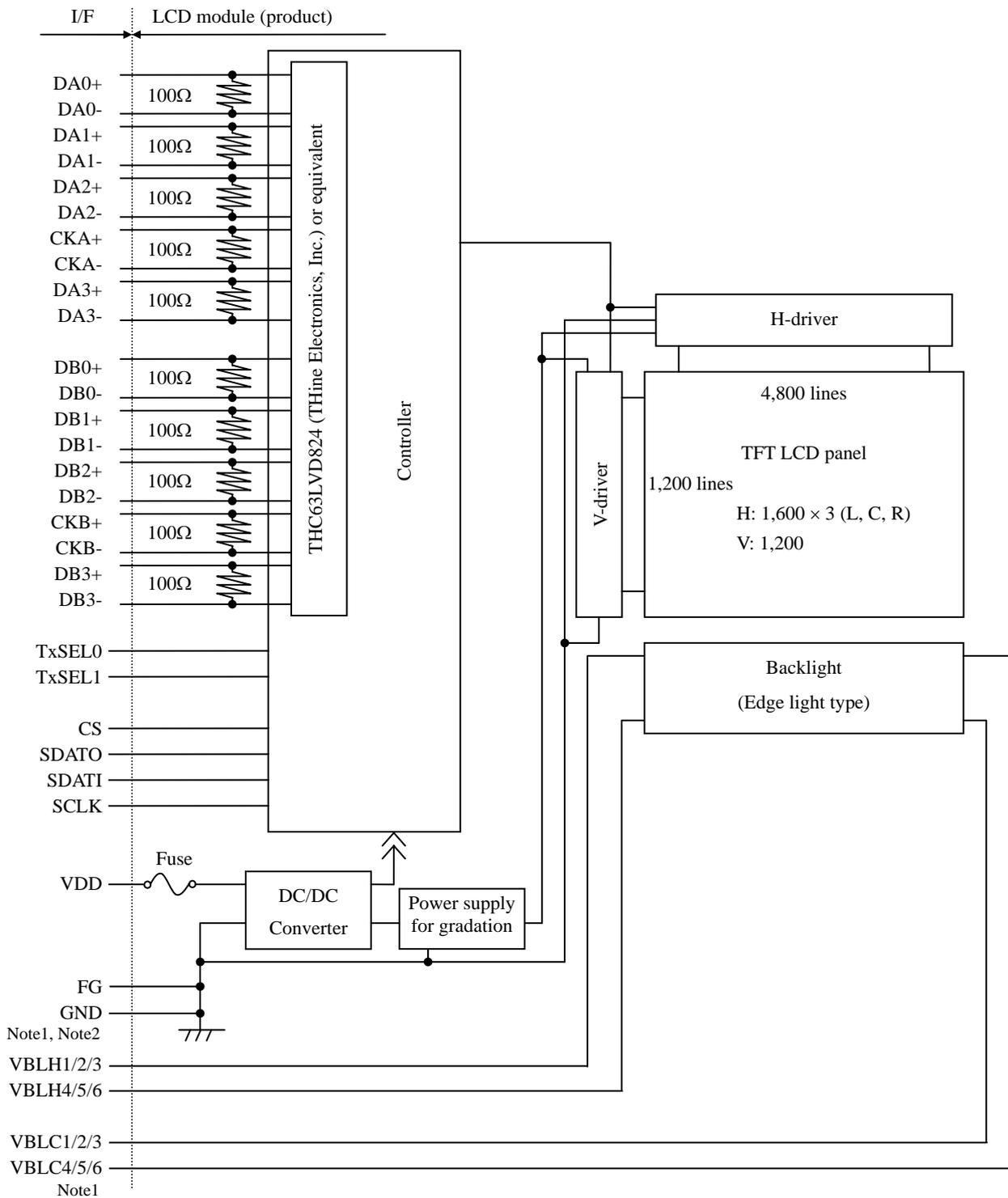
Note1: Connections between GND (Signal ground), FG (Frame ground) and VBLC (Lamp low voltage terminal) in the product
