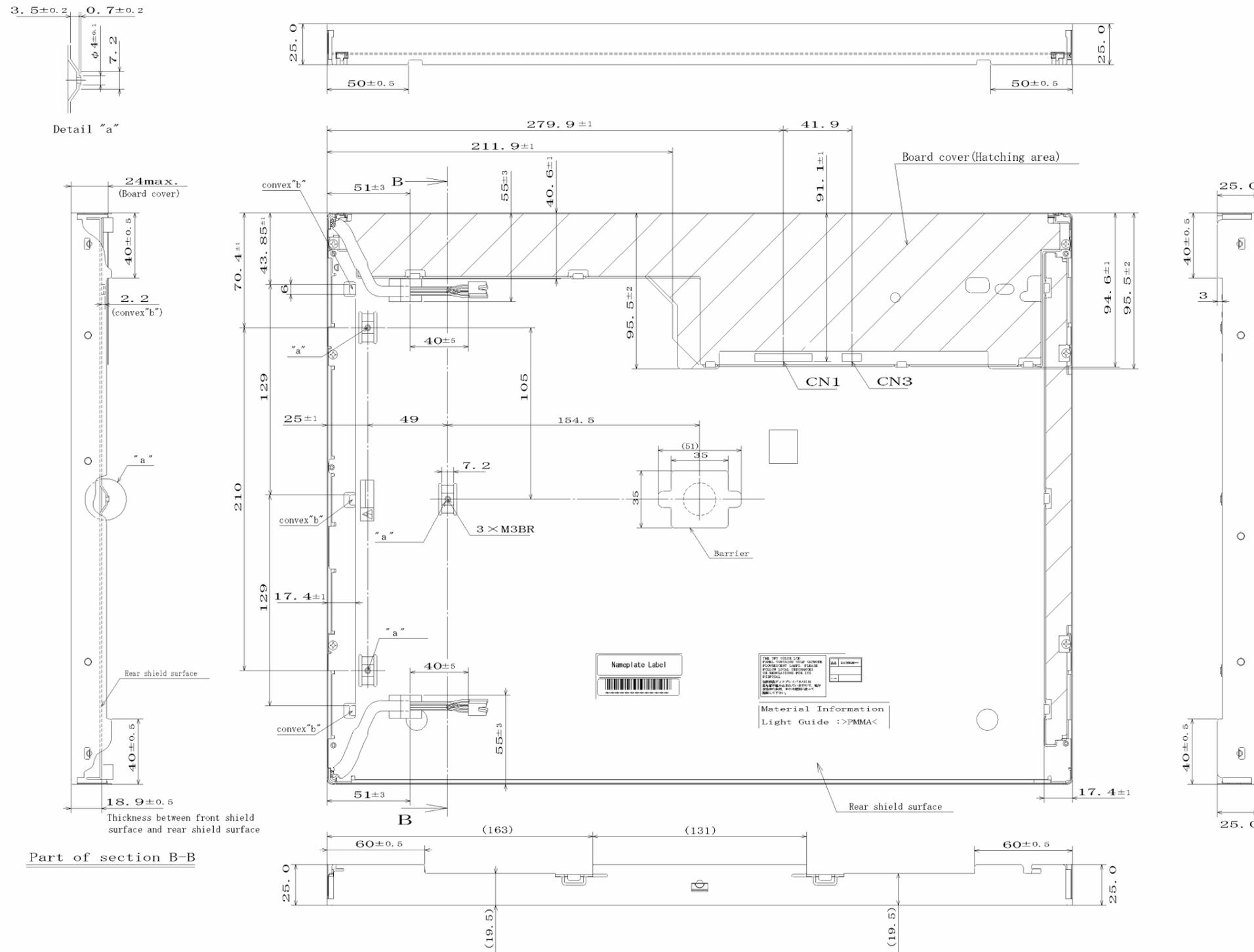
Note1: Not shown tolerances of the dimensions are  $\pm 0.5 \text{ mm}$ .
