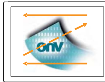
Fig. 2 Reverse scan (Pin19, RSV = High or VDD)
