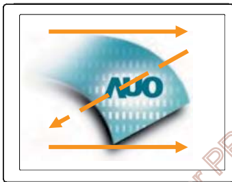
Fig. 1 Normal scan (Pin19, RSV = Low or NC)
